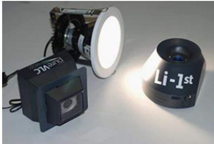
Figure 5.2.5.1 Li-1st from left ceiling unit, LED lamp and desktop unit (photoreceiver).
