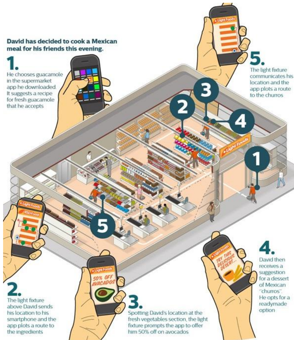
Picture 5.2.3.1: example of how the Philips smart lighting system works [17].
